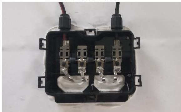
Inside view of Junction box
